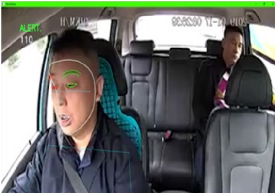
Fig. 4: Algorithm Detecting Alertness in Driver
